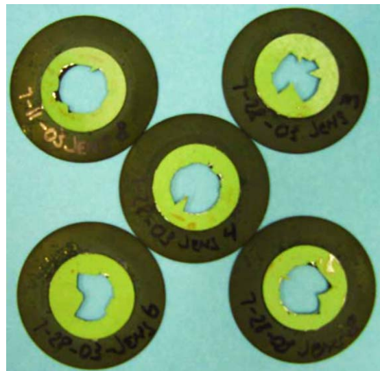
Fig. 3. Examples of specimen failure upon rupture testing.
